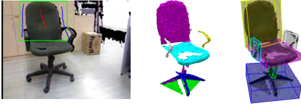
Fig. 3 Initial proxy generation. The user is allowed to scribble strokes on the image (left), and based on the scribbles, depth-augmented GrabCut is applied to segment the input object to different parts (middle). Initial cuboids are then fitted to the corresponding points (right).
